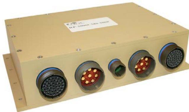
Figure 4. Solid State Power Controller Module
