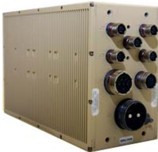
Figure 3. Electromechanical Relay/Circuit Breaker System Box
