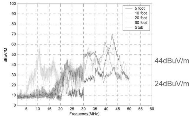
*Figure 7. Emissions on various lengths of cable*
