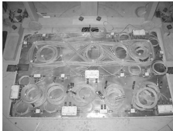
*Figure 5. 1553 network on copper ground plate*
