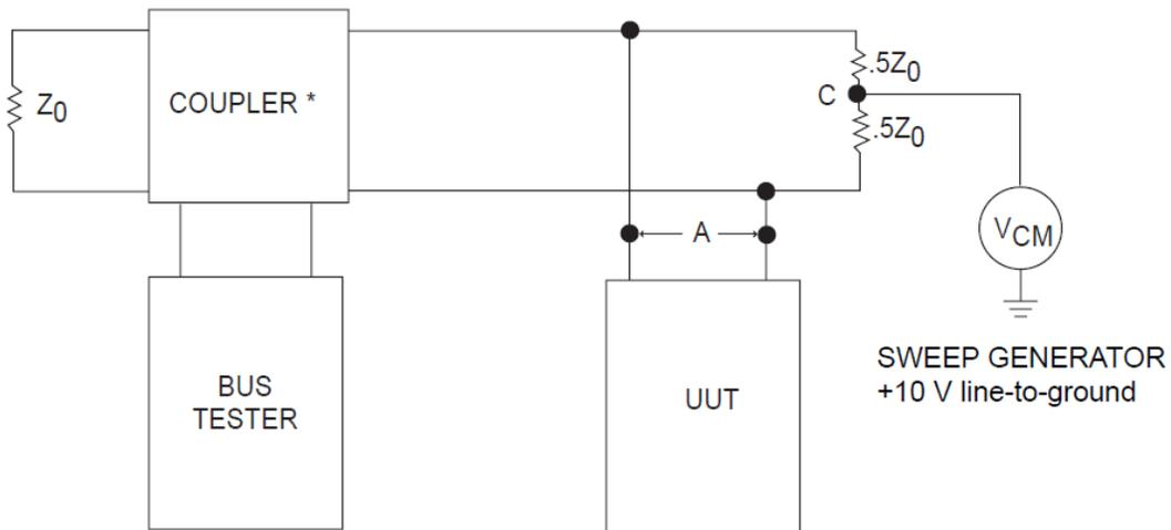
\* Transformer Coupled Stub Must Be Used
