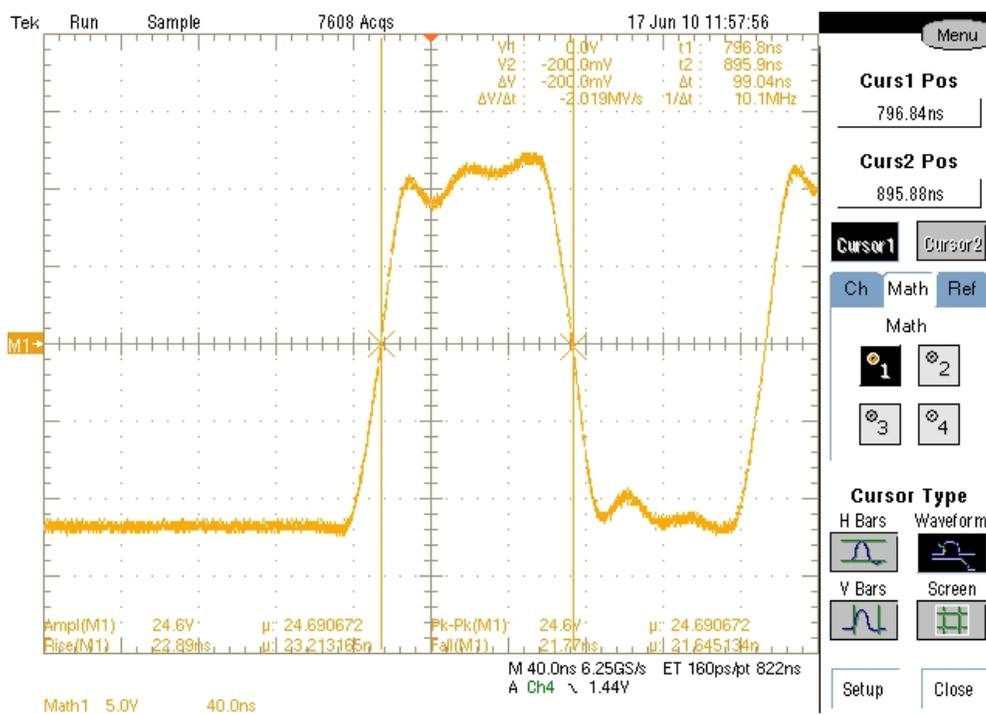
Figure 5. Zero Crossing Stability of 5 Mbps Manchester Coded Data
