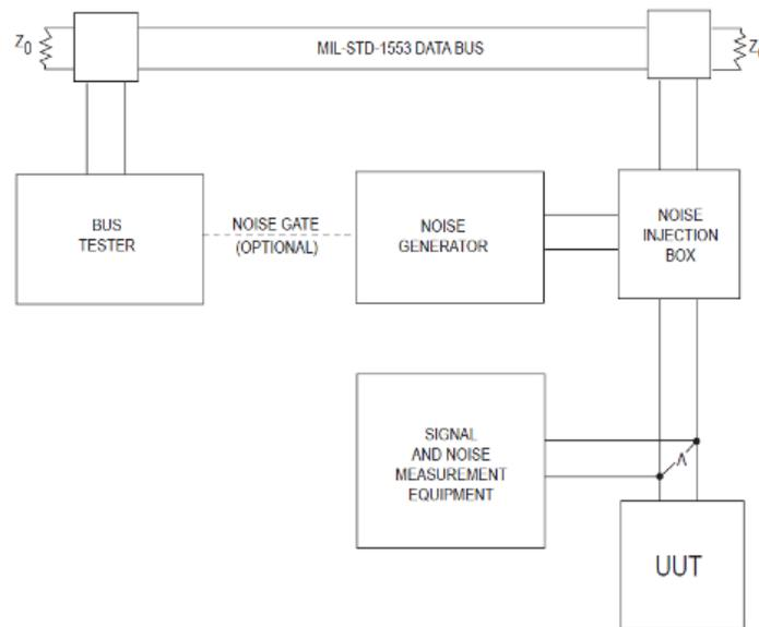
**Figure 8. Noise Rejection (Bit Error Rate) Test**
