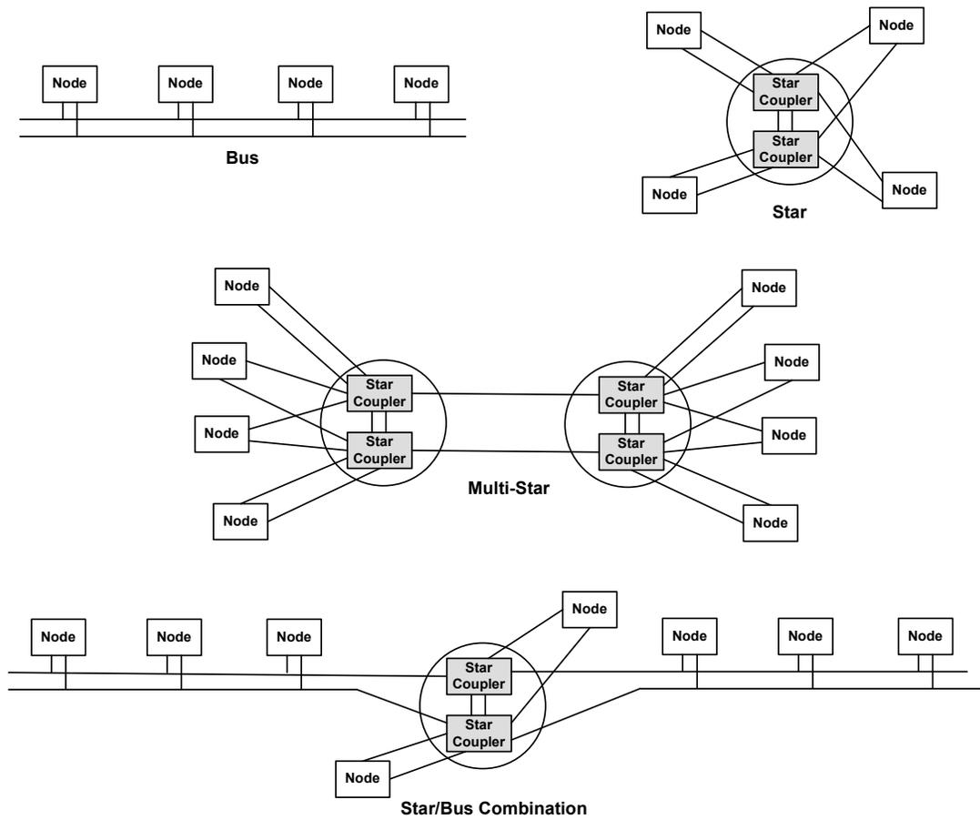
**Figure 1. TTP Topologies: Bus, Star, Multi-Star, and Star/Bus Combination<sup>1</sup>**
