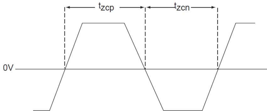
**Figure 5. Zero-Crossing Distortion**
