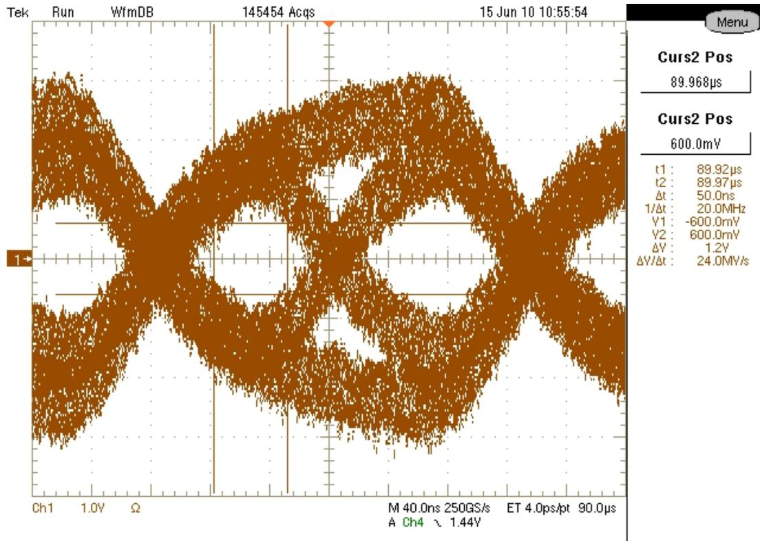
Figure 12. Eye Diagram for Powernode #7 on 430 Foot Bus with -78 dBm/Hz Noise
