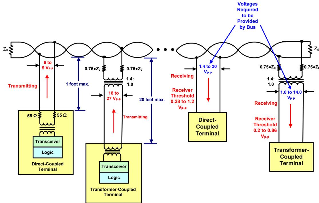
**Figure 6. MIL-STD-1553 Bus, Stub, and Receiver Voltages**
