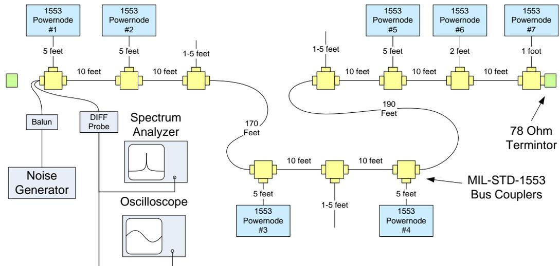
Figure 10. 430 Foot Test Bus
