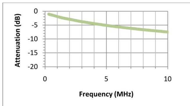
*Figure 1. Frequency Response of 300 Feet of 1553 Cable*
