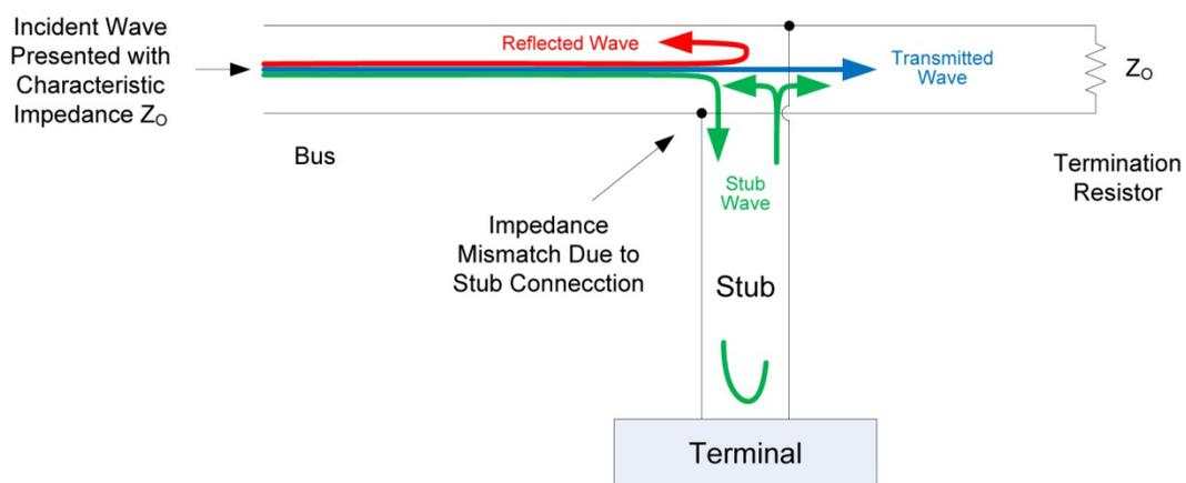
Figure 3. Reflections Caused by Impedance Mismatch
