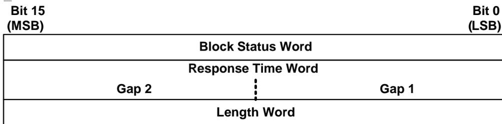
Figure 5. MIL-STD-1553B Intra-Packet Data Header
