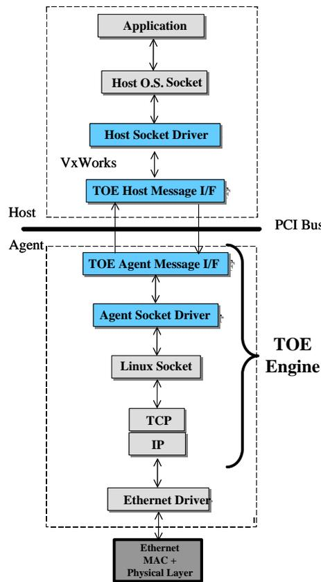
Figure 10. Stack Diagram for Gigabit Ethernet TOE Adaptor
