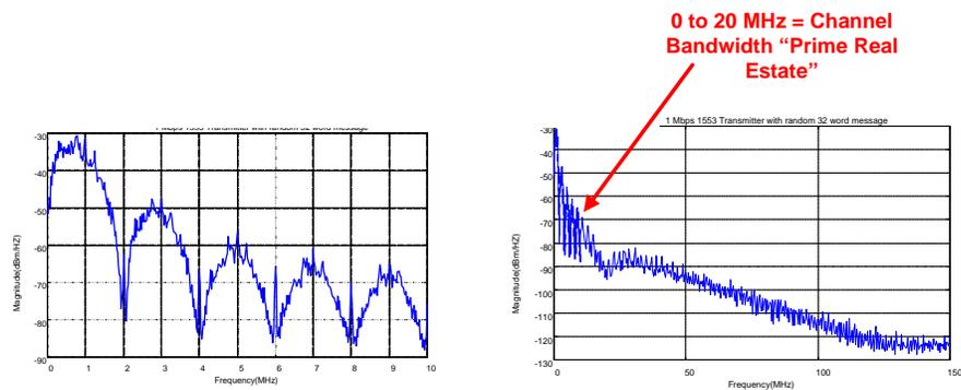
*Figure 5. Frequency Spectrum of 1 Mb/s MIL-STD-1553 Signal
