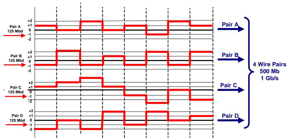
Figure 9. 1000BASE-T Gigabit Ethernet 4D-PAM5 Encoding
