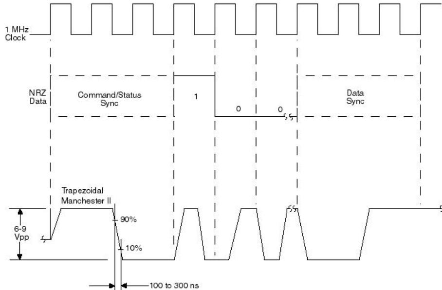
*Figure 2. MIL-STD-1553 Data Encoding and Waveshaping*
