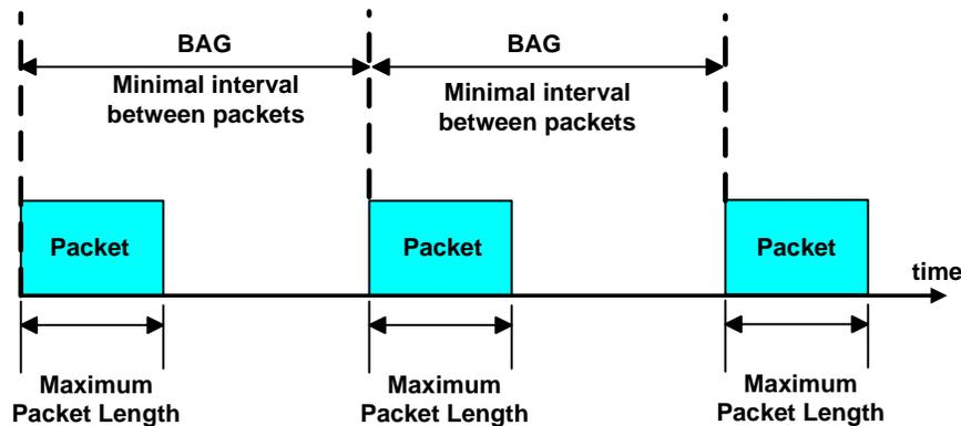
Figure 12. AFDX BAG (Bandwidth Allocation Gap)
