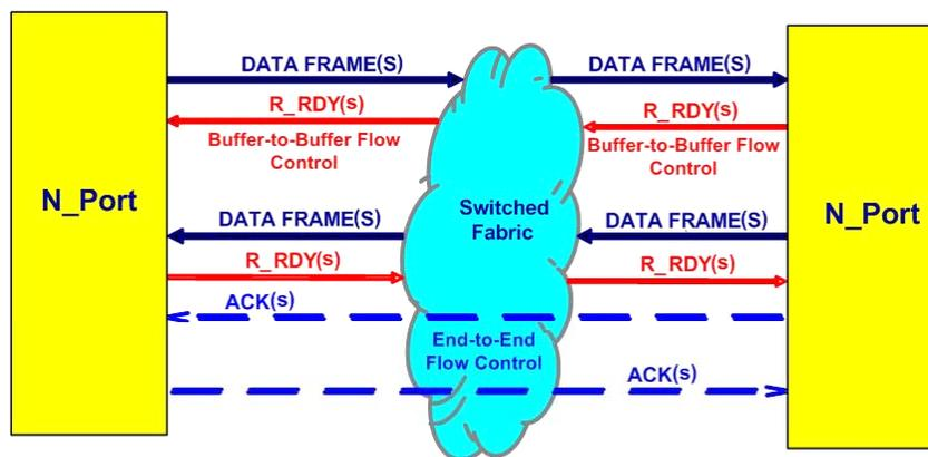
*Figure 7. Fibre Channel Buffer-to-Buffer and End-to-End Flow Control*
