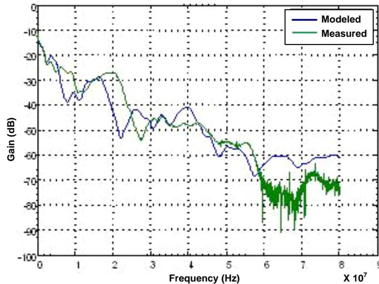
*Figure 4. Modeled and Measured Response of 1553 Bus Channel*
