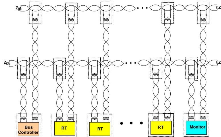
Figure 1. MIL-STD-1553 Dual Redundant Bus
