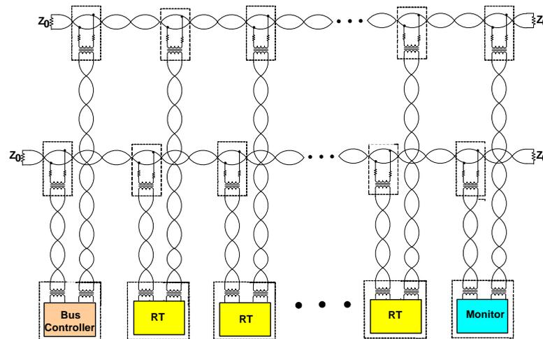
Figure 1. MIL-STD-1553 Dual Redundant Bus
