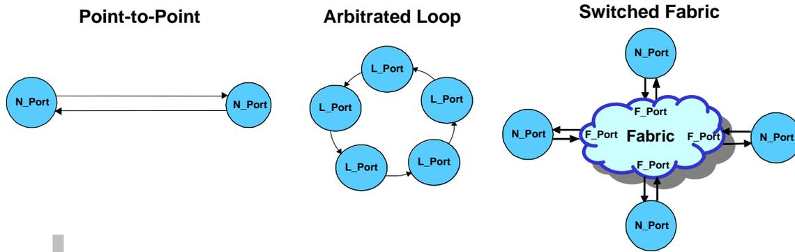
Figure 6. Fibre Channel Topologies: Point-to-Point, Arbitrated Loop, and Switched Fabric
