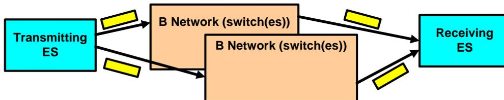
*Figure 11. AFDX Redundancy*
