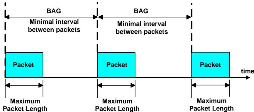
Figure 12. AFDX BAG (Bandwidth Allocation Gap)
