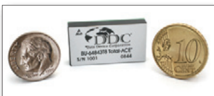
Figure 4. Fully integrated 1553 terminal DDC Total-ACE
